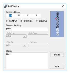
Enter a device IP address and SNMP credentials and click "Submit" to test communications. The tool will attempt to ping the remote device to see if it responds to a ping before doing the SNMP query.
