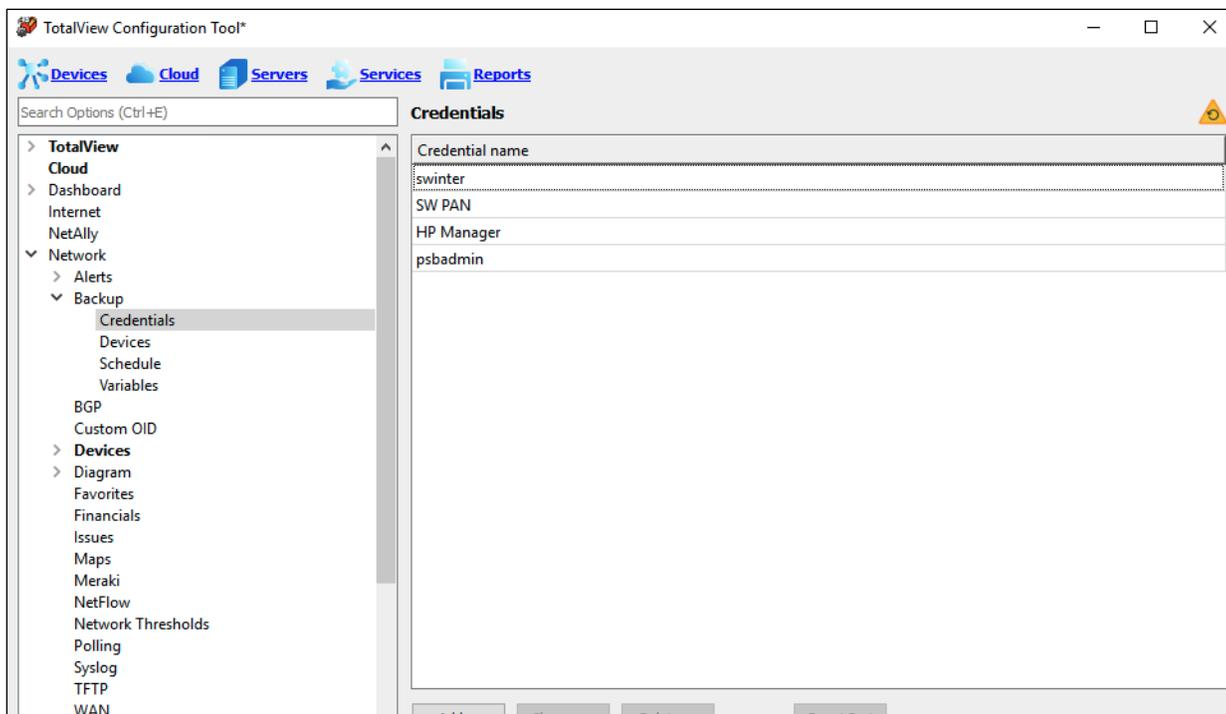
Select **Add** to add credentials to the system. The dialog box asks you to enter the username and password that you would use for SSH connect to a switch or router. Typically, this would be your Radius server credentials or a set of credentials created on the system for TotalView to use.
