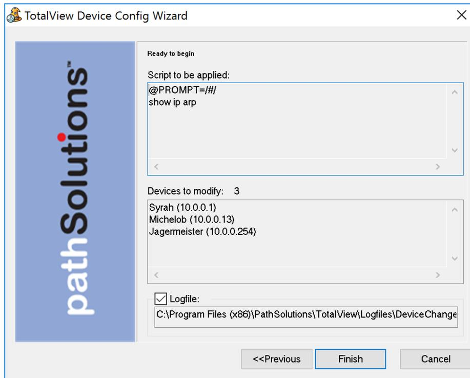
The wizard will then start applying the configuration query to the devices and show a status of each. When completed, it will open the device change log to show the results of each communication.
