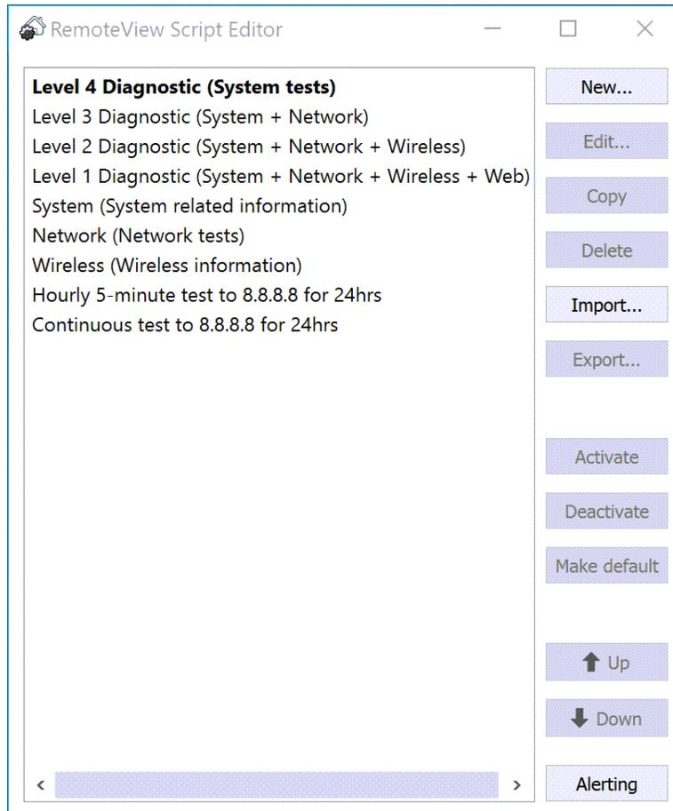
To edit a script, select the script (the Level 4 Diagnostic is shown below), and select **Edit**. A dialog box will appear that allows you to name and describe scripts, the place that script results are logged, and what tests the script performs. You can also setup notes and notifications.
