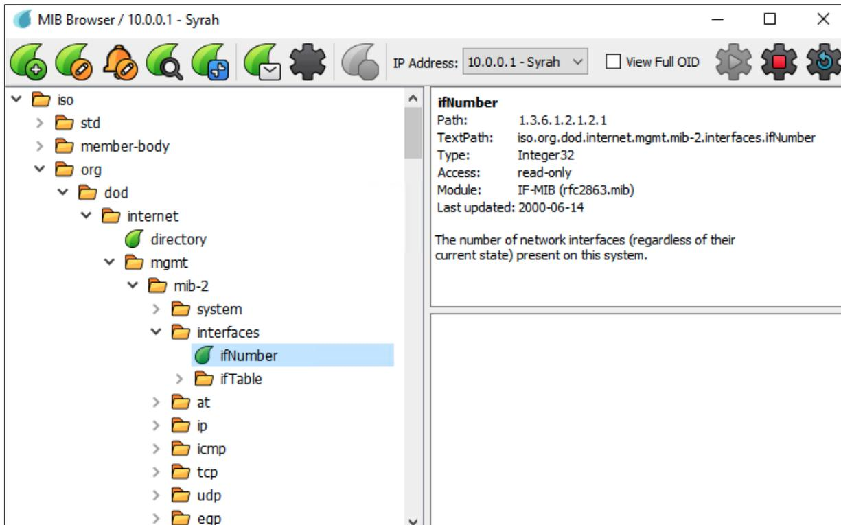
Most all manufacturer's MIBs have been automatically added into the database so variables can be immediately queried without the need to find and compile MIBs. Live and historic graphing and tracking of variables are also available to see inflection changes.
